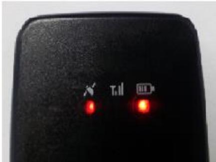
It is highly recommended that the rechargeable battery should be charged completely before using the device. Connect the ST940 to its charger cable supplied by Suntech and charge it for 5 hours.
