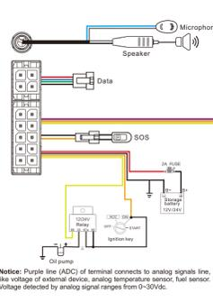
**Notice:** Purple line (ADC) of terminal connects to analog signals line, like voltage of external device, analog temperature sensor, fuel sensor. Voltage detected by analog signal ranges from 0-30Vdc.
