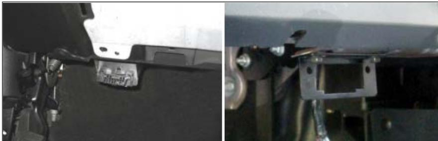
Figure 10: Vehicle OBD-II Port Connector and OBD-II Flange Mounted
