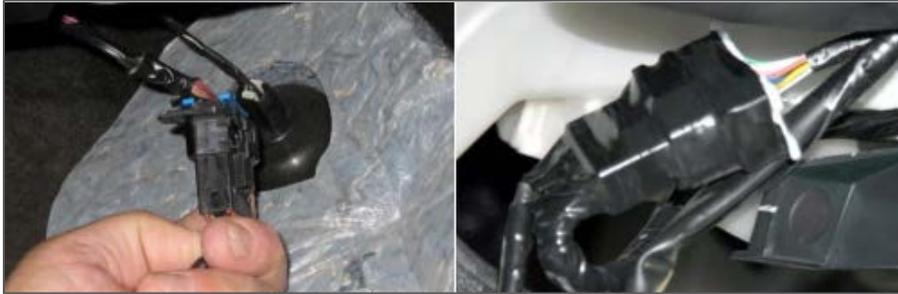
Figure 11: Plugged OBD-II Connectors and Taped Connectors
