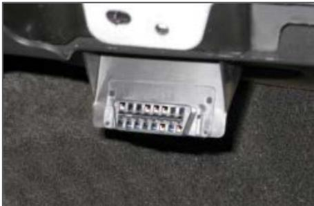
Figure 12: Re-mounted OBD-II Port Connector
