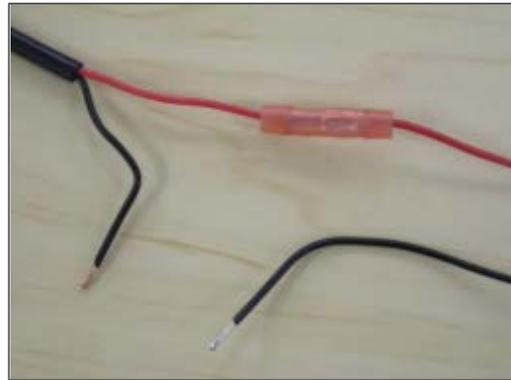
Figure 9: Connect Power and Ground using supplied connectors
